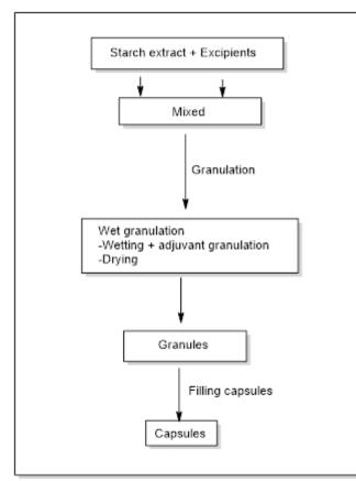
Figure 1. Main stages of wet granulation
